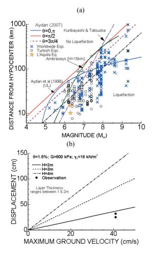
Figure 16. Comparison of observations with estimations from the method proposed by Aydan et al. (2008) based on maximum ground velocity.
