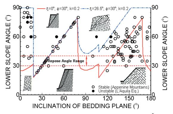
Figure 14. Comparison of observational data with computational results prom previous studies ( $\xi$ : intermittency angle; *k*: horizontal seismic coefficient;  $\phi$ : friction angle).
