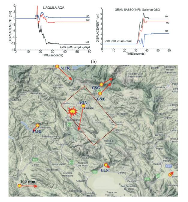
Figure 11. (a) Estimated ground movements during earthquake at selected points, and (b) estimated permanent ground displacements by EPS method.
