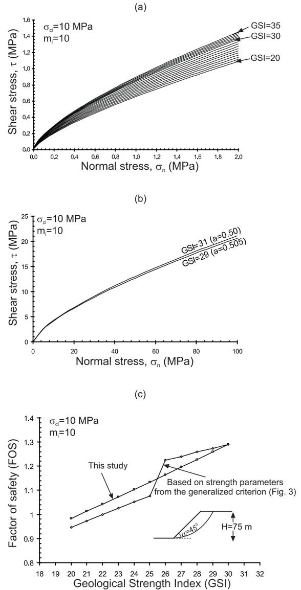
Figure 10. Applications of the improvements suggested in this study to the Hoek-Brown criterion: (a) failure envelopes for the GSI values between 20 and 35 without any strength gap, (b) failure envelopes of two rock masses constructed by assuming a switch GSI value of 30, and (c) comparison of the 'FOS-GSI' plots derived from this study and the generalized criterion for the hypothetical slope shown in Figure 2.
