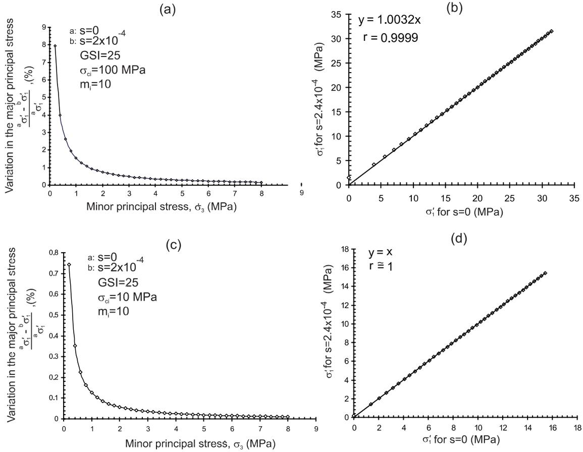
Figure 7. Variation in the major principal stress in terms of  $s=0$  and  $s=2.4 \times 10^{-4}$  with minor principal stress (GSI=25).
