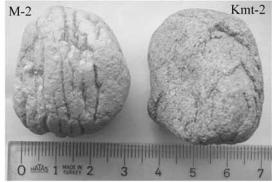
Şekil 4. İkinci çevrim sonunda tamburda kalan (a) marn (M-2) ve (b) kumtaşı (Kmt-2) örnekleri ve bu örneklerde gelişen zayıflık düzlemleri. Figure 4. A view of the M-2 (a) and Sst-2 (b) test specimens in the drum at the end of the second cycle, and weakness planes that developed in these specimens.
