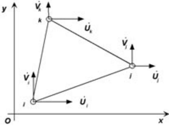
Figure 1. Coordinate system and the definition of displacement rates for a triangular element.
