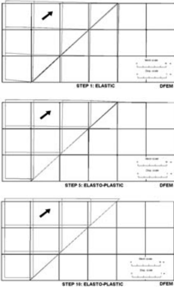
Figure 8. Deformed configurations during various computation steps.
