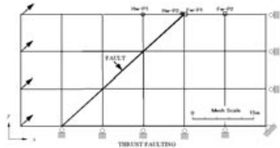
Figure 7. Finite element mesh used in DFEM analysis.
